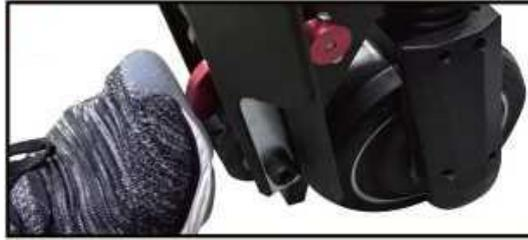
Check that the scooter looks to be ok Be sure that the valve is open and press on the red handle.
